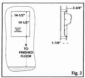
Begin with a 14-1/2" W  $\times$  19-1/2" H rough wall opening framed on all sides. Make sure the opening is the correct distance above the floor. Refer to the chart below for mounting heights.
