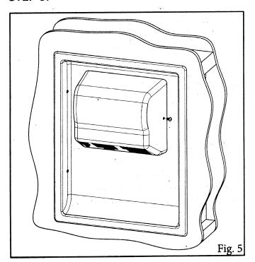
Place cover on dryer and secure with (2) tamper proof security screws (included with dryer). Turn power on at breaker and test.
