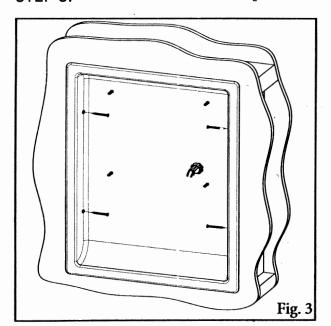
Insert the recess box into the rough wall opening. Run electrical through conduit entrance as shown. Using the provided wood screws, secure recess box to wall studs as shown in figure 3.
